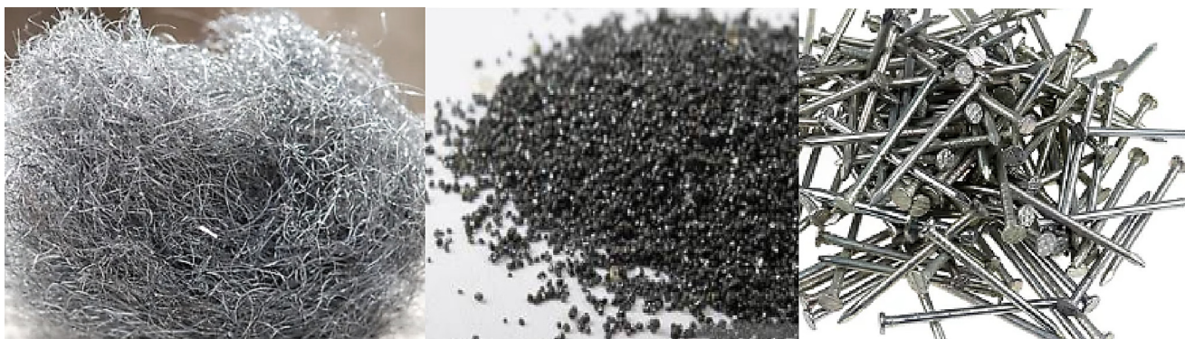
Fig. 2. Iron wool, iron fillings and iron nails used in experiments.
