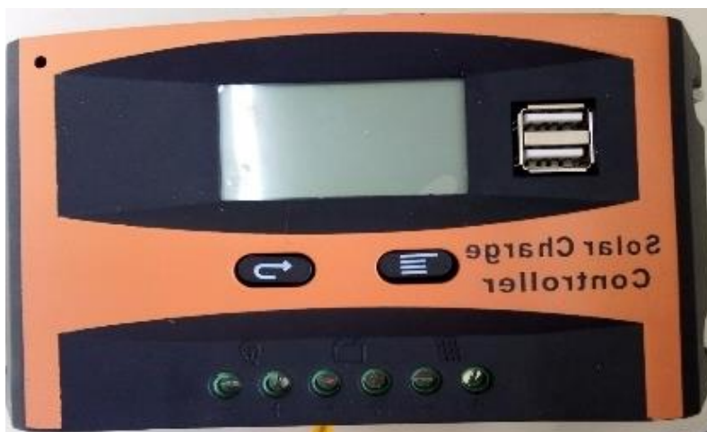
Figure 6: Solar charge controllers
