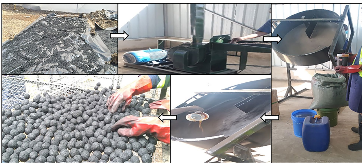
Fig. 5 Illustration of the briquette-making process after carbonization
