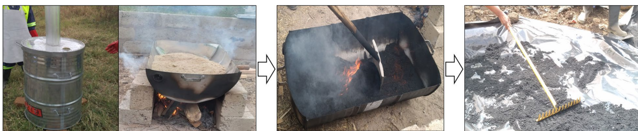
Fig. 4 Carbonization process of faecal sludge by manually made carbonization furnace and sawdust in an open drum (1st two images from left) followed by cooling process and sorting (3rd and 4th images from left)
