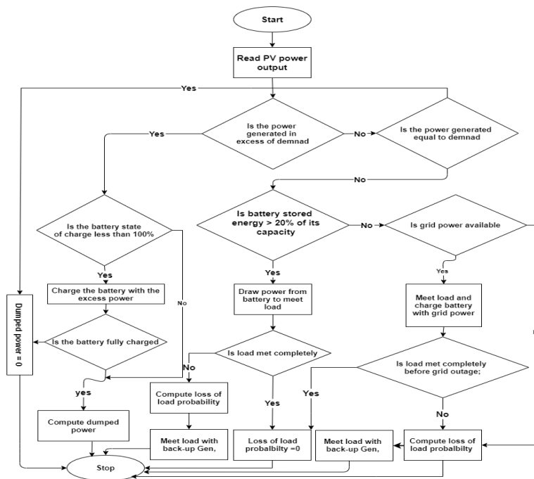
Figure 3. Detailed control logic and the modelled energy management strategy.
