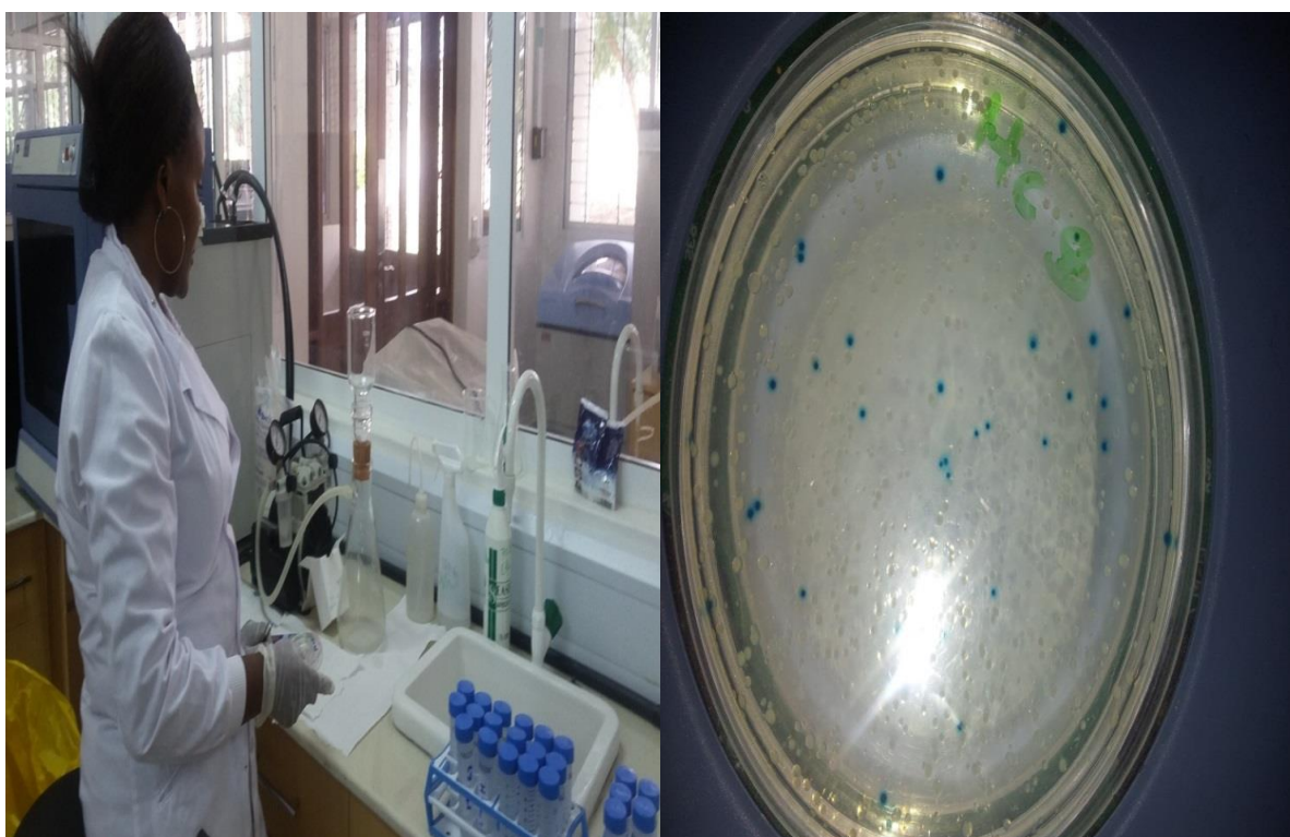
Figure 15: To the left, membrane filtration, to the right E. coli blue colonies from fresh milk samples
