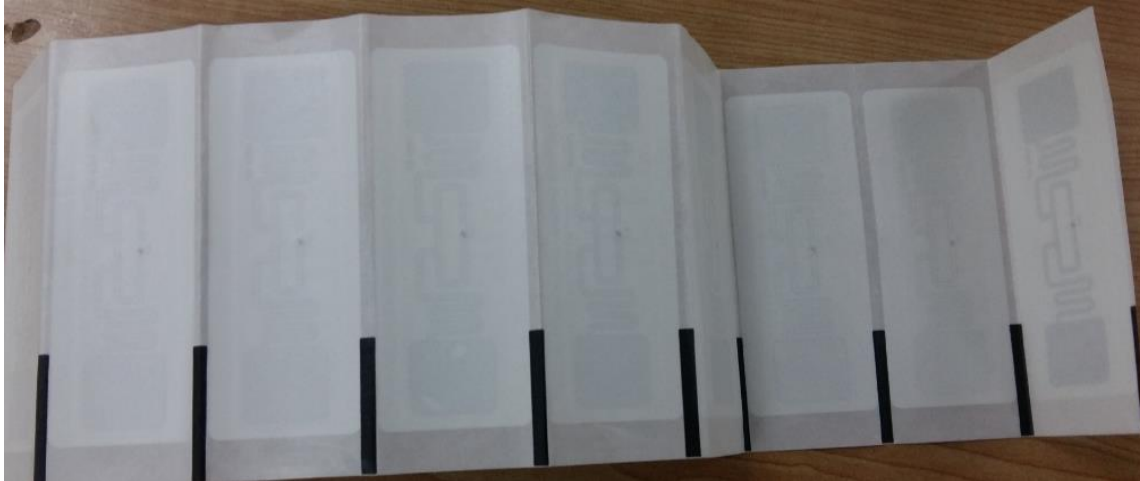
Figure 11: Alien UHF adhesive tags
