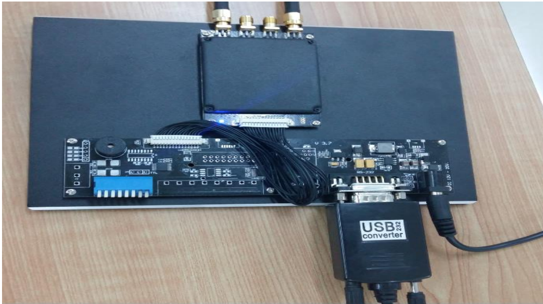
Figure 12: 4 ports RFID reader
